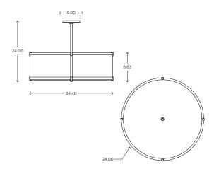
The Litebox combines subtle elements of classical style with a respect for contemporary simplicity. The result is a fixture that complements almost any architectural space. It is available in custom sizes, levels of trim (with or without crossbars), as a flush mount or pendant, and with custom finishes, diffusers, and lamping.
