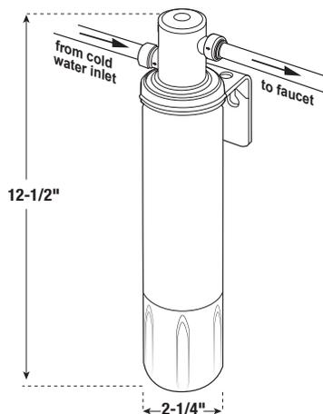
**F-1000 Cartridge (included with this system) Chemical & Mechanical Reduction Filter Specifications:**
