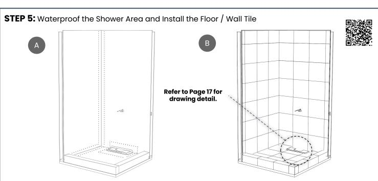
Install waterproofing membrane to all areas required. Apply sealing compound and strip seals along the reservoir's edges to ensure it is adequately adhered to the prefabricated shower base. This will provide a water-tight seal. Install floor and wall tiles when ready using a  $\frac{1}{2}$ " x  $\frac{1}{2}$ " U-shaped trowel. Tile thickness should be within **8 to 12mm** to ensure proper alignment of the RainStick to its reservoir. **Refer to page 16 for further details.**
