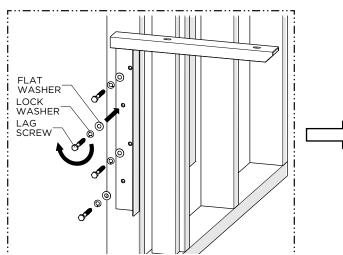
Install the BRACKETS using the LAG SCREWS and WASHERS provided.
