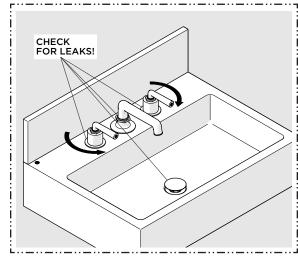
12. Turn on the water and operate the drain and faucet [sold separately] to ensure proper operation. Check all connections for leaks. If desired, a bead of caulk or clear silicone may be applied where the SINK contacts the finished wall.
