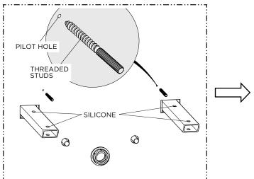
7. Install the M8 THREADED STUDS making sure the wood end is fully inserted into the finished wall then apply adhesive silicone to the top surfaces of the SUPPPORT BRACKETS.
