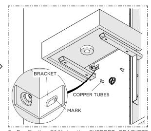
Dry-fit the SINK to the SUPPORT BRACKETS ensuring it is level and re-adjust or shim (not included) if necessary. Mark the hole locations for the ANGLE BRACKETS. Remove the SINK and drill pilot holes for the M8 THREADED STUDS provided.
