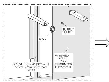
Ensure the SUPPLY LINES and DWV STUB OUT are properly installed and all the required blocking is in place then complete the FINISHED WALL installation.
