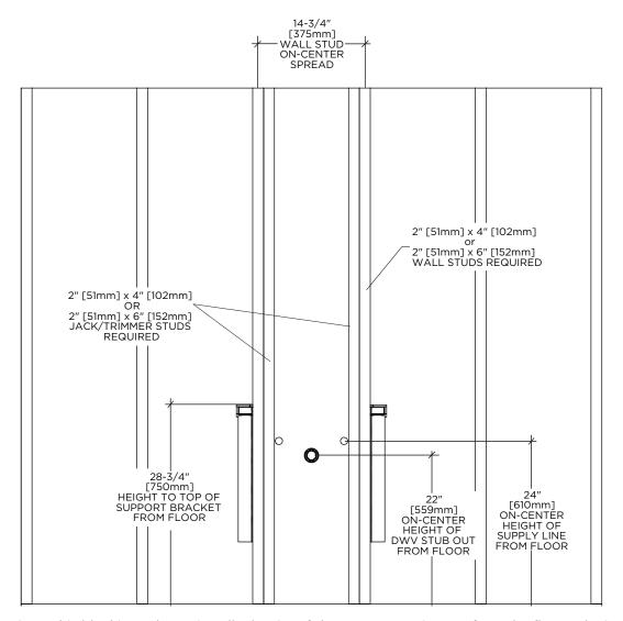
**NOTE:** This blocking scheme installs the rim of the SINK 34" [864mm] from the floor. Take into account the sub-floor and finished floor material thickness to obtain the desired height.
