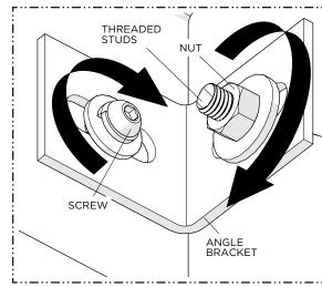
If necessary, cut the excess length from the THREADED STUDS then securely and evenly tighten the NUTS and SCREWS to secure the ANGLE BRACKETS.
