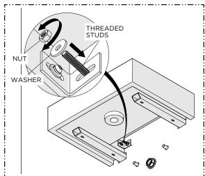
8. Place the SINK on top of the BRACKETS and push it against the wall making sure the silicone does not wipe off. Remove any excess silicone around the SINK. Install the WASHERS and NUTS provided onto the THREADED STUDS and hand-tighten.
