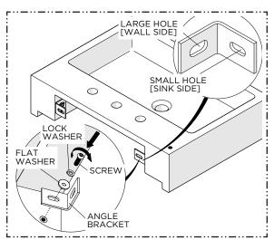
5. Install the ANGLE BRACKET to the underside of the SINK using the SCREWS and WASHERS PROVIDED. Do NOT tighten the SCREWS.
