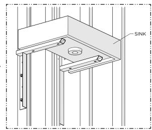
Dry-fit the SINK to the BRACKETS to ensure the weight of the SINK is properly supported then remove the SINK and keep it properly stored until final installation.
