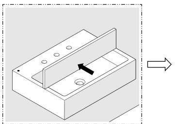
10. If desired, install the BACKSPLASH provided using an adhesive silicone.
