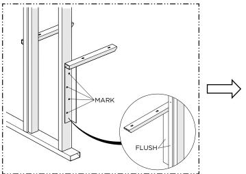
Dry-fit the BRACKETS to the WALL STUDS and mark the location of the mounting holes. Make sure to hold the BRACKETS level and flush with the front face of the STUDS. Drill pilot holes for the 3/8" [10mm] LAG SCREWS provided.
