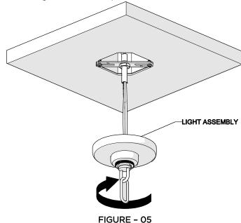
14. Thread the LIGHT ASSEMBLY to the NIPPLE on the MOUNTING PLATE making sure it's secure.
