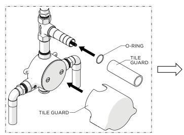
4. Install the TILE GUARDS to protect the VALVE during the completion of the finished wall and to create the exact opening for access to the SERVICE STOPS and future servicing.
