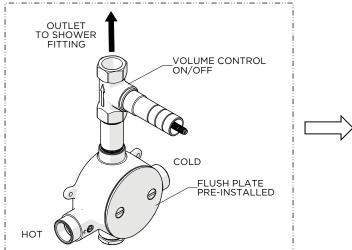
Make sure the VALVE is positioned according to the markings so that the inlets are situated with hot piped on the left and cold piped on the right.
