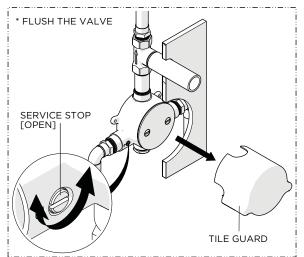
5. Turn on the water supply, remove the TILE GUARD, and open the SERVICE STOPS to flush out the lines to prevent the FILTER SCREENS from clogging.
