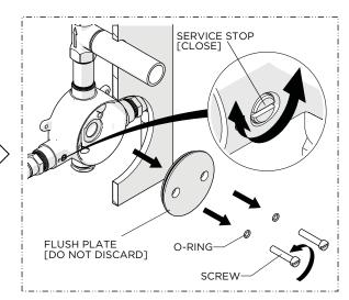
6. After flushing, turn off the water supply, close the SERVICE STOPS, unthread the SCREWS, and remove the FLUSH PLATE [Do NOT discard].
