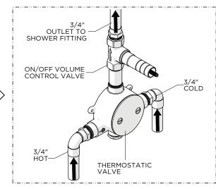
3. Run 3/4" COPPER SUPPLY lines to the proper height of the VALVE inlets and be sure to secure all piping and fittings.
