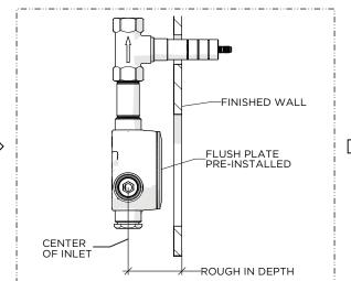
The VALVE rough-in depth is measured from the center of the inlets to the surface of the finished wall and varies depending on the trim being used.
