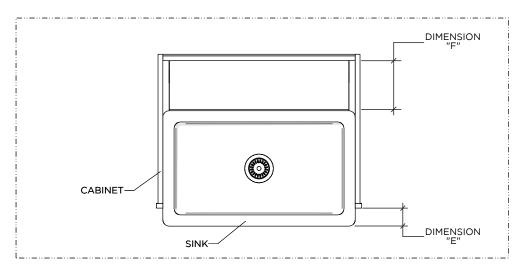
Position the sink so that the apron or front of the sink projects out of the cabinet as desired, DIMENSION "E", and there is enough room between the sink and the back of the cabinet, DIMENSION "F", for the faucet fittings.
