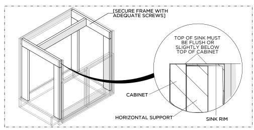
4. Ensure that the supports are secured using SCREWS (not provided) and level.
