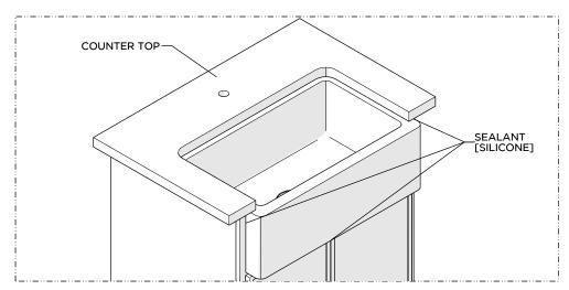
10. Apply a bead of silicone sealant where the sink contacts the countertop and cabinet surfaces. Remove any excess sealant.
