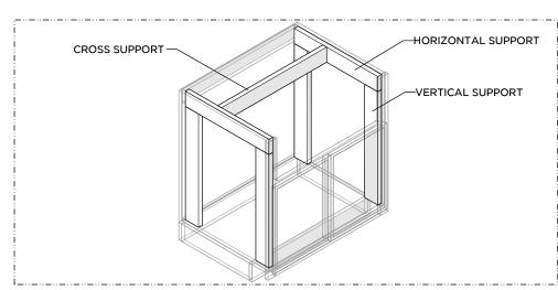
3. Using adequate support framing material, install a support frame inside the CABINET that will securely support the weight of the SINK. **EXAMPLE:** A support frame may consist of 2 horizontal supports, 4 vertical supports, and a cross support.
