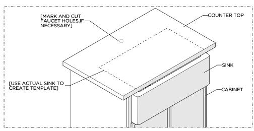
With the SINK in the final position, create a template to transfer onto the countertop then cut the countertop per manufacturer's instructions and cut the faucet hole(s) prior to final installation.
