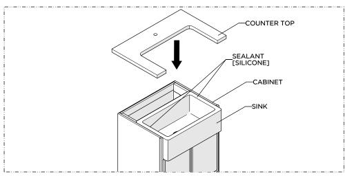
9. Apply a bead of silicone sealant to the back and sides of the SINK then place the countertop on top of the cabinets.
