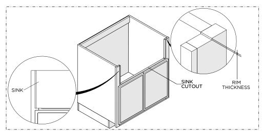
2. Place painter's tape on the front surface of the CABINET and trace the shape of the SINK onto the tape. Cut the CABINET along the line drawn.
