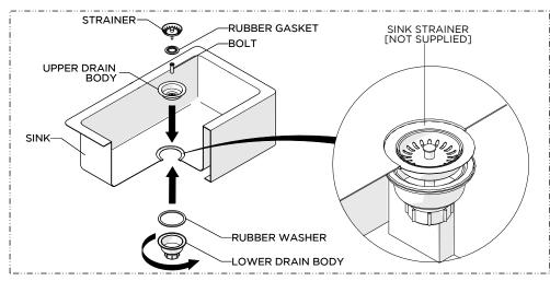
5. Install the strainer onto the SINK, per the manufacturer's instructions
