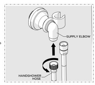
3. Thread and securely tighten the knurled end of the HOSE to the ELBOW.
