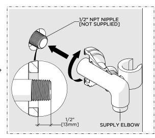
2. Ensure the 1/2" NPT NIPPLE (not supplied) projects 1/2" [13mm] from the surface of the finished wall then thread and securely tighten the SUPPLY ELBOW onto the NIPPLE.
