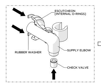
Slide the ESCUTCHEON and RUBBER WASHER onto the SUPPLY ELBOW.
