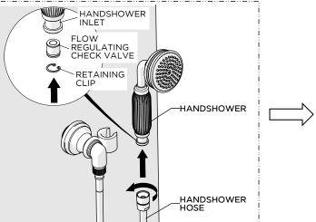
5. Thread and securely tighten the conical end of the HOSE to the HANDSHOWER.
