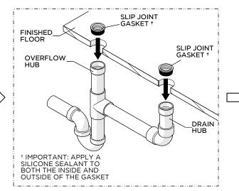
11. Apply a generous coating of a clear adhesive silicone sealant to both the **inside** and **outside** of the SLIP JOINT GASKETS and insert the GASKETS into the DRAIN HUBS.
