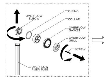
Unthread and remove the SCREW, OVERFLOW GRILL, OVERFLOW GASKET, COLLAR, and O-RING. Remove OVERFLOW RISER PIPE from OVERFLOW ELBOW.
