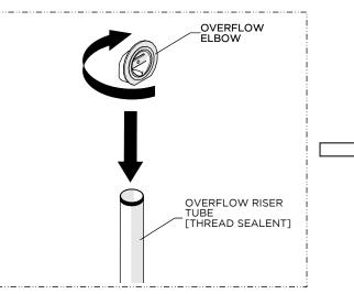
8. Apply thread sealant or pipe dope to the threads on the RISER TUBE then thread and securely tighten the ELBOW onto the TUBE.
