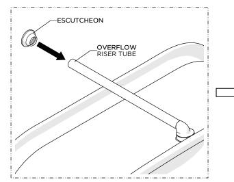
10. Slide the ESCUTCHEON onto the OVERFLOW RISER TUBE.
