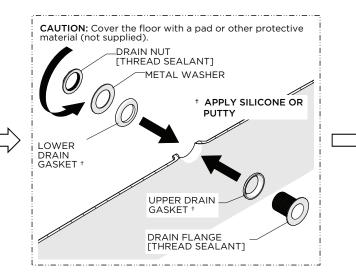
5. With the BATHTUB on its side, apply a **generous** bead of silicone or putty to the UPPER and LOWER GASKETS and set the FLANGE then thread and securely tighten the NUT onto the FLANGE.
