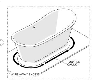
15. Run a bead of tub and tile caulk around the bottom edge of the BATHTUB where it meets the finished floor and wipe away any excess caulk with a wet paper towel.
