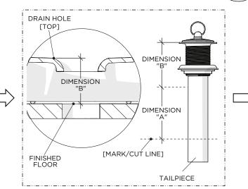
2. Measure (DIMENSION "B") from the top of the DRAIN HOLE to the finished floor then, using the previous DIMENSION "A", mark and cut the DRAIN TAILPIECE.
