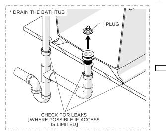
14. Drain the BATHTUB and inspecting all connections above and below the finished floor for leaks where possible if access is limited.
