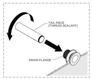
6. Thread the TAILPIECE into the DRAIN FLANGE.
