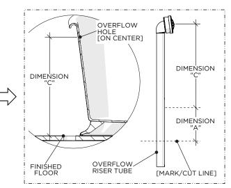
3. Measure (DIMENSION "C") from the center of the OVERFLOW HOLE to the finished floor then, using the previous DIMENSION "A", mark and cut the OVERFLOW RISER TUBE.
