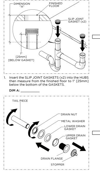
4. Remove the STOPPER, UPPER and LOWER DRAIN GASKETS, WASHERS, NUT and TAILPIECE from the DRAIN FLANGE.
