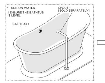
Verify the BATHTUB is level and, if needed, add shims then fill the BATHTUB until water enters the overflow hole.
