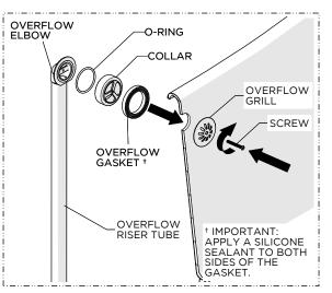
Apply a generous bead of silicone sealant to both sides of the OVERFLOW GASKET then assemble the OVERFLOW RISER TUBE to the BATHTUB making sure to include the COLLAR and O-RING and securely tightening the SCREW.
