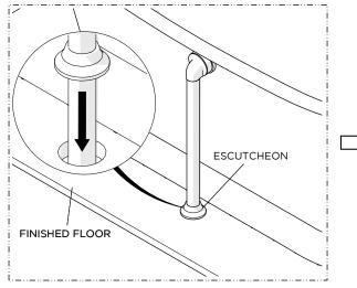
16. Slide the ESCUTCHEON down the OVERFLOW RISER TUBE until it contacts the finished floor.
