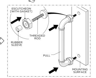
2. Pre-assemble the ESCUTCHEONS and RUBBER SLEEVES onto the THREADED RODS on the PULL then insert the RUBBER SLEEVES into the predrilled holes.
