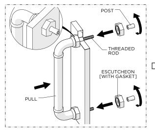
3. Slide the ESCUTCHEONS onto the THREADED RODS then thread and securely tighten the RETAINING POSTS.
