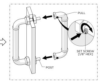
4. Slide the 2nd PULL onto the RETAINING POSTS until it contacts the ESCUTCHEONS then thread and securely tighten the SET SCREWS.
