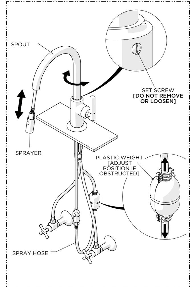
9. Pull out the SPRAYER and rotate the SPOUT to ensure the PLASTIC WEIGHT can move freely beneath the cabinet.
