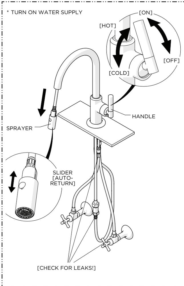
7. Turn on the water supply and operate the HANDLE and SPRAYER to ensure they function properly and to flush out any debris in the supply lines then check all connections for leaks and turn off the water.
