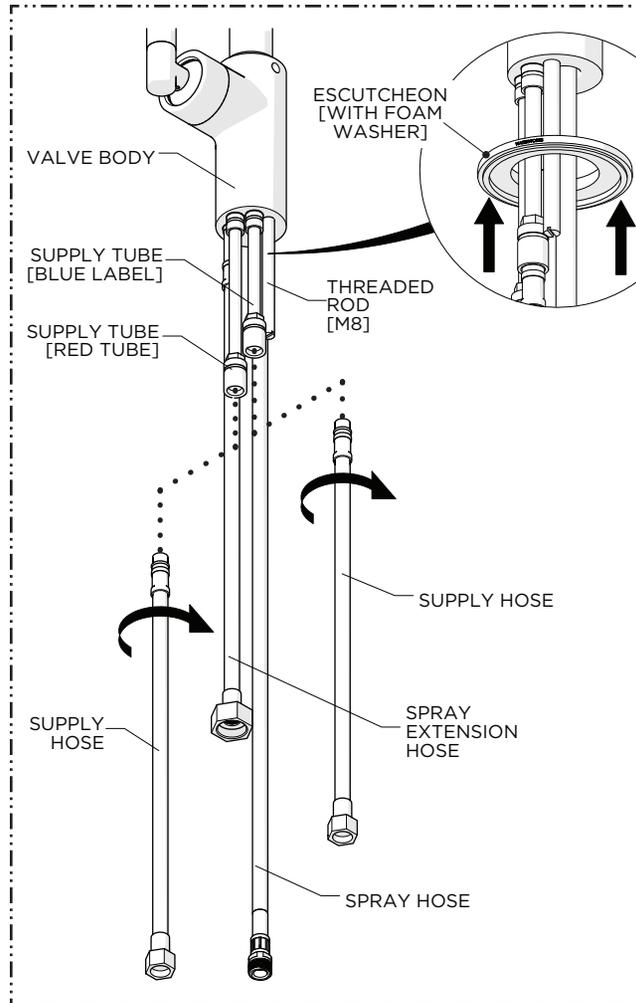
2. Thread and securely tighten the SUPPLY HOSES into the SUPPLY TUBES on the VALVE BODY then slide the ESCUTCHEON (with FOAM WASHER) over all HOSES, TUBES, and THREADED ROD.
