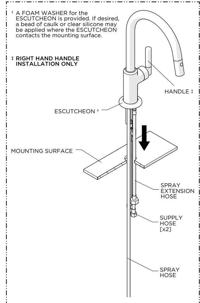
† A FOAM WASHER for the ESCUTCHEON is provided. If desired, a bead of caulk or clear silicone may be applied where the ESCUTCHEON contacts the mounting surface.
