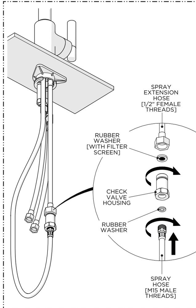
5. Connect the SPRAY HOSE to the EXTENSION HOSE using the CHECK VALVE HOUSING and RUBBER WASHERS provided.
