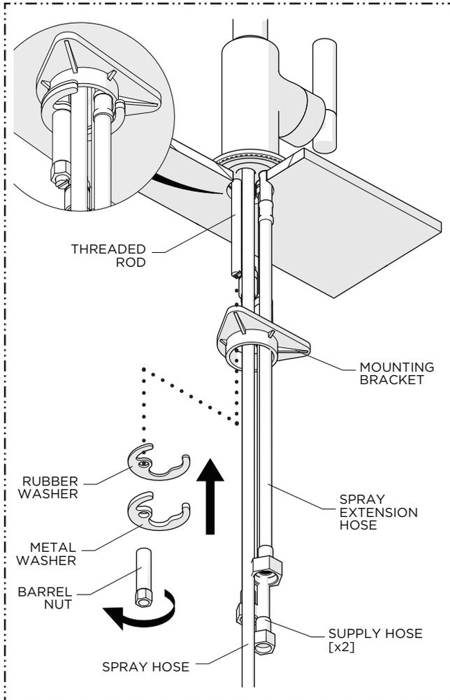
4. Slide the MOUNTING BRACKET over the HOSES and THREADED ROD and place the WASHERS onto ROD then thread and securely tighten the BARREL NUT onto the ROD.
