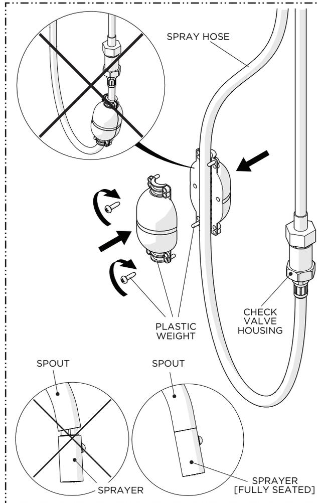
8. Attach the PLASTIC WEIGHT to a **straight** section of the SPRAY HOSE that is opposite the CHECK VALVE HOUSING and **verify** that the SPRAYER seats properly into the SPOUT.
