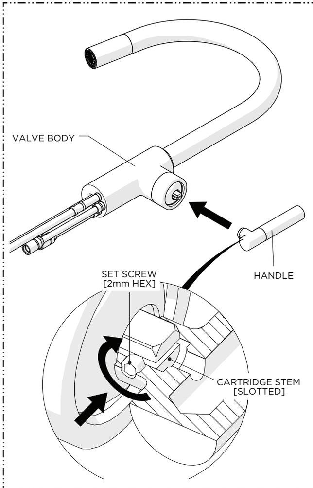
1. Slide the HANDLE onto the CARTRIDGE STEM until it is fully seated then securely tighten the SET SCREW at the base of the HANDLE.
