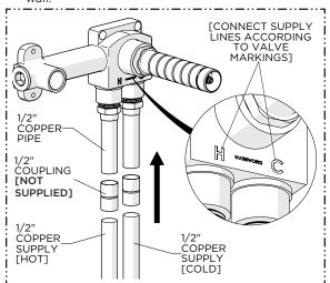
4. With the VALVE in the desired orientation, run 1/2" copper supply lines to the appropriate height and depth then connect to the VALVE using 1/2" COUPLINGS (not supplied). Make sure the hot and cold supplies are piped according to the VALVE markings.
