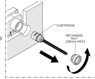
2. Unthread and remove the RETAINING NUT then pull the CARTRIDGE out of the VALVE BODY.
