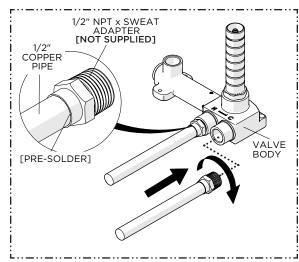
Pre-solder 1/2" COPPER PIPE to two 1/2" MALE NPT x SWEAT ADAPTERS (not supplied) then thread the ADAPTERS into the VALVE BODY.
