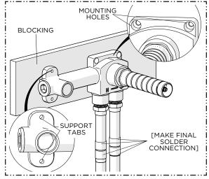
Verify the supplies are secure, level, and at the proper spread of 1-3/16" [30mm] prior to making final sweat connections. If necessary, utilize the SUPPORT TABS and MOUNTING HOLES on the VALVE to secure it to blocking or other support material using appropriate SCREWS (not supplied).
