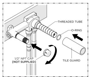
7. CAP the 1/2" NPT NIPPLE and attach the TILE GUARD to the THREADED TUBE until construction is completed.
