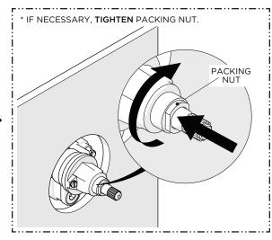
The PACKING NUT needs to be securely tightened to prevent a water leak from the CARTRIDGE STEM and create adequate rotational friction to maintain HANDLE position.
