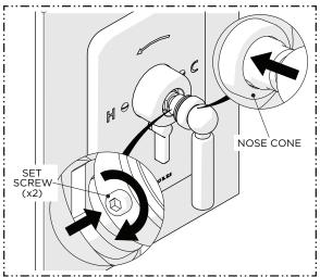
13. With the HANDLE fully seated, securely tighten the SET SCREWS (x2) then push the NOSE CONE into the GLAND COVER.
