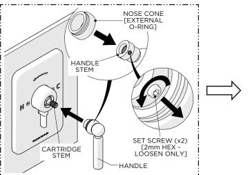
12. Slide the NOSE CONE over the HANDLE STEM then loosen the SET SCREWS (x2) and attach the HANDLE to the CARTRIDGE STEM.
