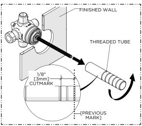
2. Remove the THREADED TUBE then cut it 1/8" [3mm] **behind** the previous mark so the TUBE will recess 1/8" [3mm] into the finished wall surface.
