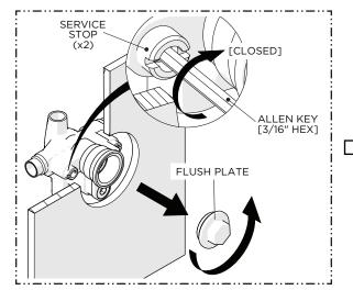
After the lines have been fully flushed, CLOSE the SERVICE STOPS (hot & cold) then unthread and remove the FLUSH PLATE.
