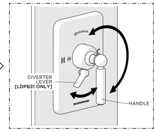
14. Operate the PRESSURE BALANCE TRIM and DIVERTER TRIM, if used, to ensure they are functioning properly.
