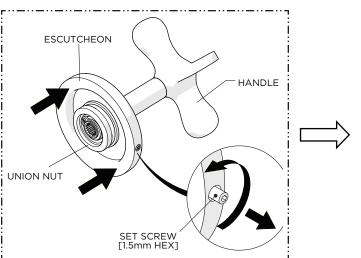
7. Loosen [do NOT remove] the SET SCREW at the base of the ESCUTCHEON then CAREFULLY slide the ESCUTCHEON up the HANDLE to expose the UNION NUT.
