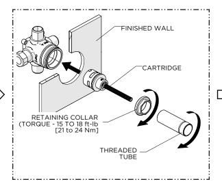
5. Re-insert the CARTRIDGE into the VALVE then thread and securely tighten the RETAINING COLLAR to the specified torque setting shown.
