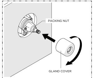
Thread and securely tighten the GLAND COVER onto the PACKING NUT.
