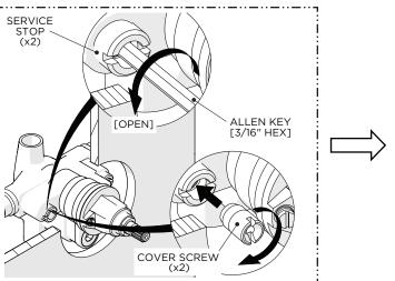
OPEN the SERVICE STOPS (hot & cold) then reinstall the COVER SCREWS (x2).
