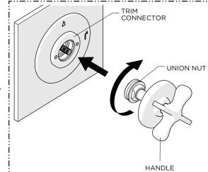
8. With the HANDLE in the desired orientation, thread the UNION NUT into the TRIM CONNECTOR until snug.
