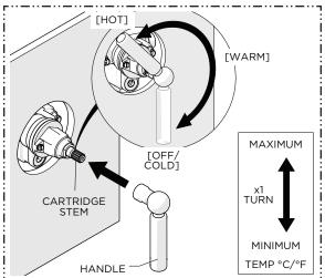
7. With the VALVE turned off, place the HANDLE on the CARTIRDGE STEM in the 6 o'clock position then turn the HANDLE counterclockwise through the cold, warm, and stopping at the hot position. Verify that a full range of temperatures exists.
