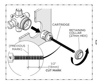
4. Unthread the RETAINING COLLAR and remove the CARTRIDGE then cut the CARTRIDGE STEM 1/2" [13mm] in front of the previous mark so the STEM will protrude 1/2" [13mm] from the finished wall surface.
