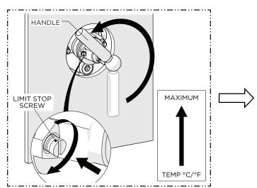
Open the VALVE to the maximum desired bathing temperature verified with a thermometer then turn the LIMIT STOP SCREW clockwise until it seats.
