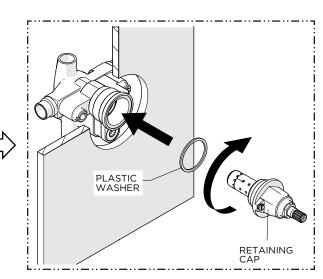
Using the PLASTIC WASHER provided, insert the CARTRIDGE into the VALVE then thread and securely tighten the RETAINING CAP.
