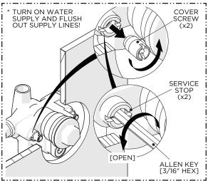
2. Turn on the water supplies then remove the COVER SCREWS (x2) and **OPEN** the SERVICE STOPS (hot & cold) to flush out the supply lines.
