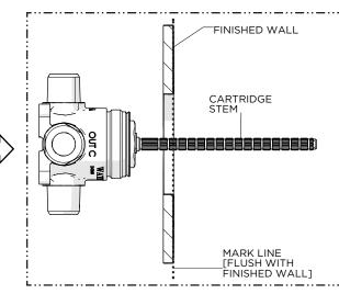
3. Mark the CARTRIDGE STEM where it protrudes past the finished wall.
