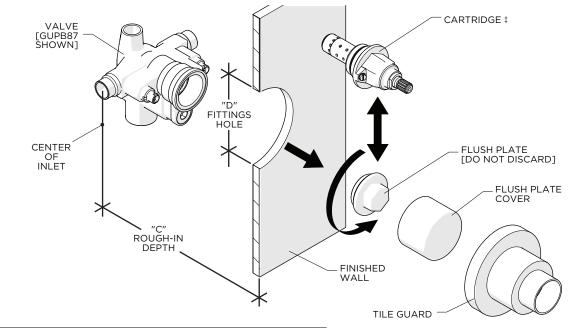
IMPORTANT: The PRESSURE BALANCE CARTRIDGE, is packaged separately and provided with the VALVE. SET ASIDE UNTIL FINAL TRIM INSTALLATION!
